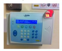
Internet to the Solihull HQ. Each employee simply touches the screen and the scanner captures the fingerprint which is compared against a stored profile to identify the employee. This is then transmitted to the central control software which then provides real time data reports tailored for specific departments.
